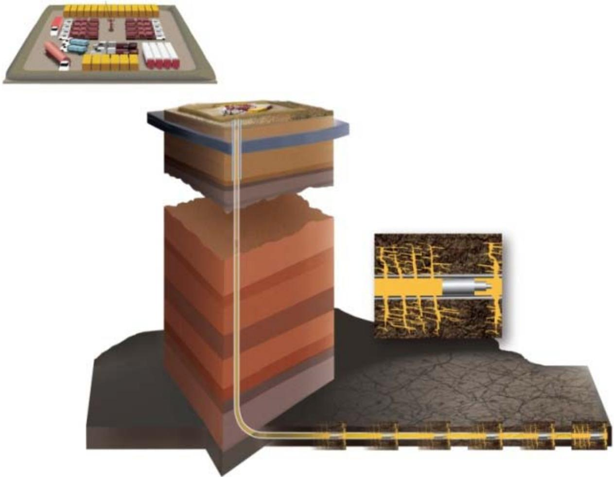
*Not to scale. The space indicated in the break between layers is usually 4,000 to 12,000 feet. If this graphic was shown with a vertical scale of 500 feet per inch (assuming a 12,000-foot-deep wellbore), this drawing would be 2 feet long!*
